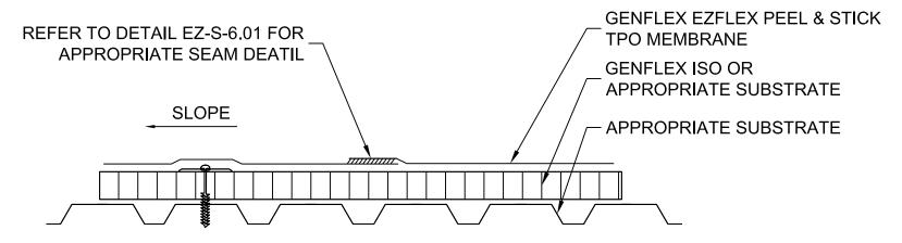
POSITION INSULATION TO ENABLE SECUREMENT INTO THE TOP FLUTES ON STEEL DECKS TO ENSURE POSITIVE ATTACHMENT AND TO REDUCE FASTENER MOVEMENT. INSULATION SHOULD BE INSTALLED WITH BOARD EDGES RESTING ON THE TOP FLUTES.
