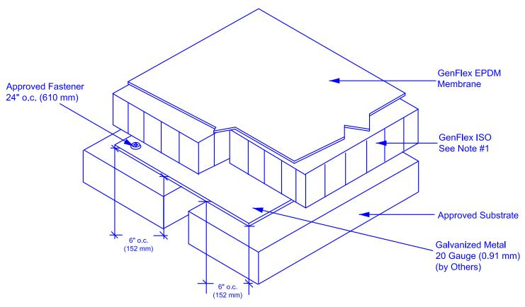
NOTE: Excessive movement due to thermal expansion/contraction may cause insulation buckling and bowing. It is the Design Professional's responsibility to determine the appropriateness of this detail.
