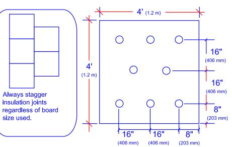
For use on buildings up to 50' (15.2 m) high. If building height exceeds 50' (15.2 m), contact the GenFlex Technical Department for attachment pattern.
