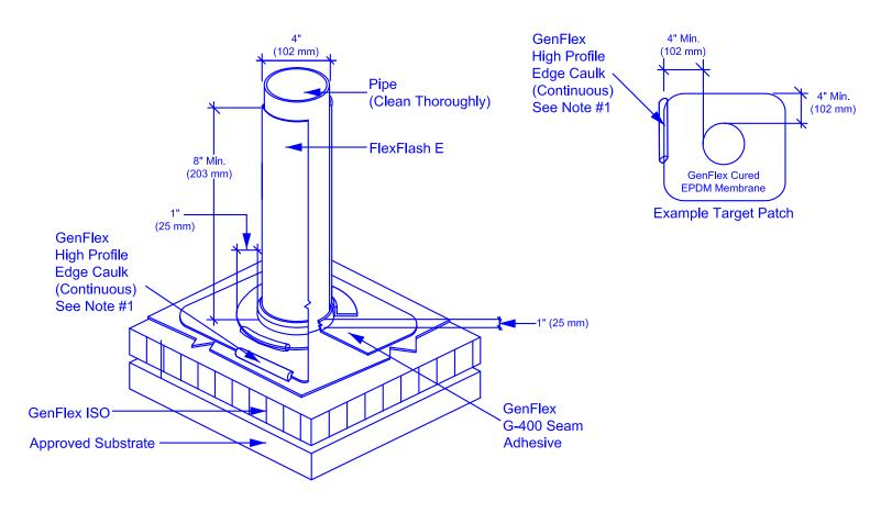
NOTE: For seams assembled with GenFlex G-400 Seam Adhesive, a bead of GenFlex Edge Caulk is required on all exposed edges, following a pre-cleaning of the seam area with GenFlex Cleaner.
