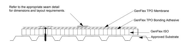
Position insulation to enable securement into the top flutes on steel decks, ensure positive attachment, and reduce fastener movement. Insulation should be installed with board ends resting on the top flutes.
