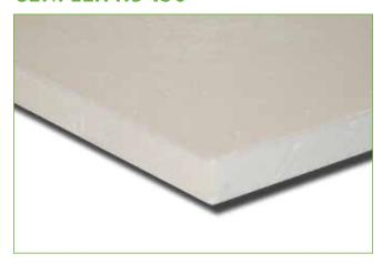
GenFlex HD ISO Cover Board is a 1/2"-thick high density cover board that incorporates several next generation features that result in a lightweight, yet extremely strong roof insulation. It combines a specially coated inorganic fiberglass facer and a high-density foam core to create a cover board that has all of the characteristics and thermal capabilities you want in an insulation.
