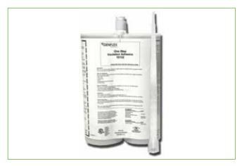
GenFlex One Step™ insulation adhesive is a highly elastic, LVOC, two component chemical curing insulation adhesive designed to adhere various roof insulations to approved decks. Each unit consists of a Part A (Isocyanurate) and Part B (Polyol) that is dispensed with a one step applicator. During the application, each component is extruded through a static mixer which blends the two components into a bead.
