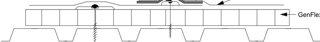
Position insulation and membrane sheets to enable securement into the top flutes on steel decks, ensure positive attachment, and reduce fastener movement. Insulation should be installed with board ends resting on the flute tops.
