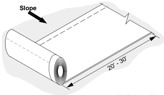
Unroll the GenFlex Peel & Stick™ membrane 20' to 30' and align as required ensuring the selvage edge of the panel is downslope to facilitate proper seam lapping (shingle lapping) in the direction of water flow. Care is required in order to ensure proper alignment of the membrane panel.
