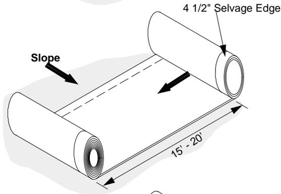
Back roll the laid out membrane 10' to 15'. The 15' to 20' of membrane left rolled out at this point is intended to keep the panel aligned. Care should be taken to avoid shifting the panel during back rolling.
