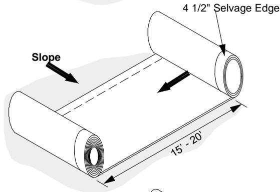
Back roll the laid out membrane 10' to 15'. The 15' to 20' of membrane left rolled out at this point is intended to keep the panel aligned. Care should be taken to avoid shifting the panel during back rolling.
