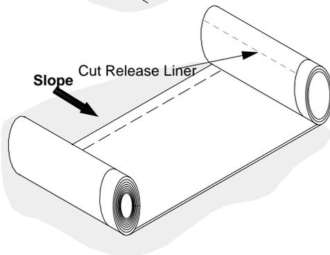
Carefully cut the release liner across the back rolled membrane as shown in the detail - **DO NOT CUT THE ROOFING MEMBRANE**. If a cut in the membrane does occur a proper repair to the membrane surface will be required following installation. After the release liner is cut, peel the edge of the release liner along the cut and proceed to pull the release liner from the adhesive film on the membrane.
