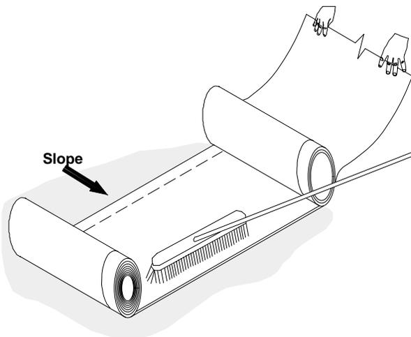
This action will also pull the membrane along the installation path as the release liner is peeled from the adhesive film. Once the roll is fully applied use a stiff bristle broom and positive downward pressure to broom in the newly applied Peel & Stick™ membrane. Brooming direction should be across the short axis of the membrane panel to avoid creating wrinkles in the sheet.
