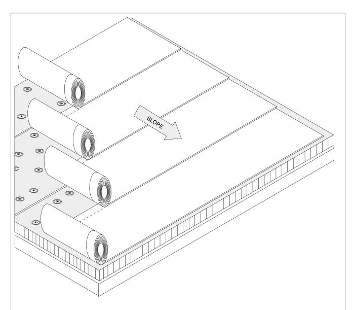
During a multiple roll apllication all seams must be shingled in the direction of water flow. Special attention is required to properly align, and maintain alignment of the GenFlex Peel & Stick™ TPO rolls during application. Refer to detail PS-16.02 Membrane Installation - Scroll Method for guidance.
