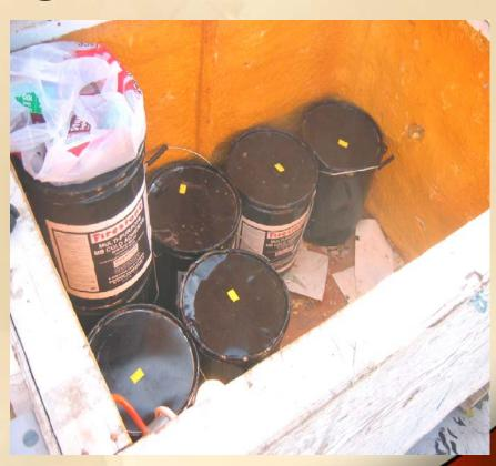
Heat provided by 100 watt light bulb inside storage box
