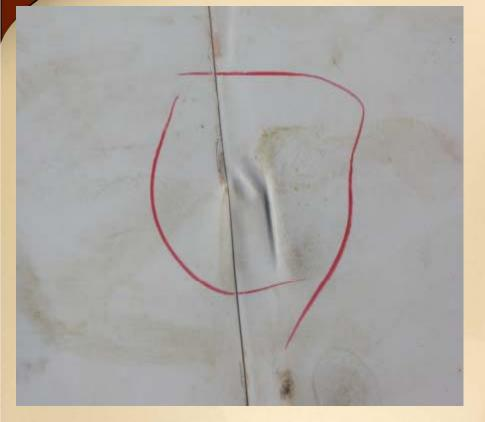
Caused by incorrect tracking and how the robot is "placed" onto the sheet. Cause by the stop of the robot and the start of hand welding.
