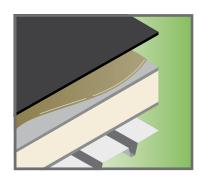
**Fully Adhered Systems** are ideal for roofs with unusual or odd-shaped contours, or where mechanical penetration of the membrane is not desirable, while providing exceptional wind performance and longevity. Once positioned over the substrate, the back of the membrane and the substrate are coated with GenFlex bonding adhesive, allowed to dry, carefully rolled back into position and broomed into place.
