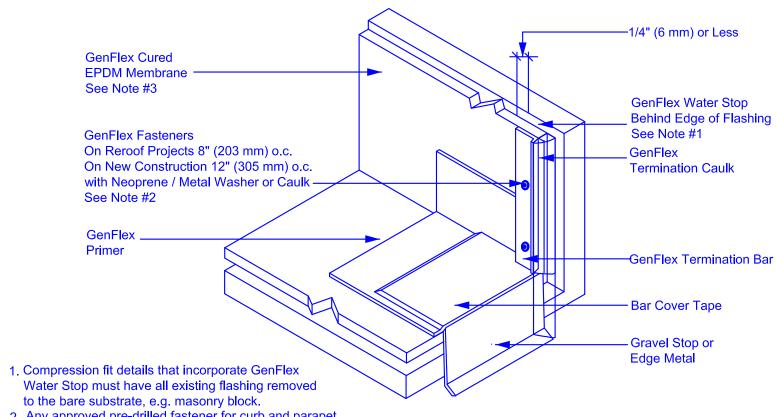
2. Any approved pre-drilled fastener for curb and parapet terminations must have a minimum 125 lb (556 N) pullout. See approved fastener list.
