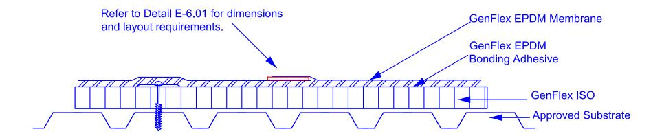
NOTE: Position insulation to enable securement into the top flutes on steel decks, ensure positive attachment, and reduce fastener movement. Insulation should be installed with board ends resting on the top flutes.
