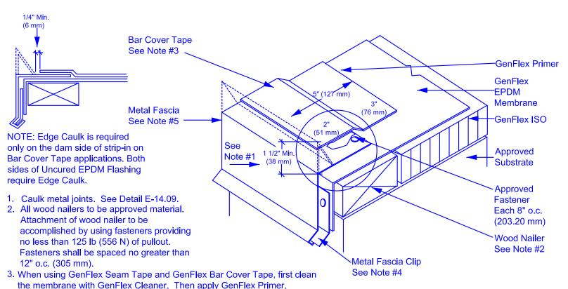
4. Metal coping cap, expansion joint, and edge details are typical only. All metalwork should be installed to sheet metal codes (SMACNA). Clean all metal prior to installation of GenFlex materials.
