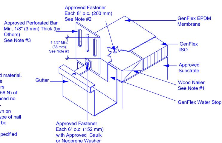
1. All wood nailers to be approved material. Attachment of wood nailer to be accomplished by using fasteners providing no less than 200lb (556 N) of pullout. Fasteners shall be spaced no greater than 12" o.c. (305 mm).
