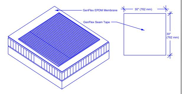
Remove the release paper from the seam tape, and mate the walkway pad to the prepared surface in a smooth motion, avoiding buckles in the walkway pad. Walk the walkway pad into place, or roll with a suitable roller.
