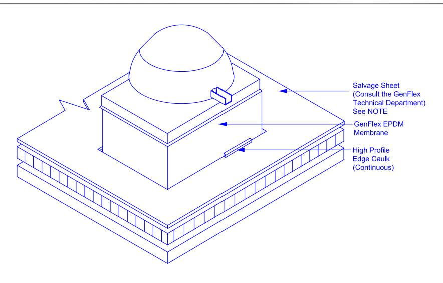
NOTE: Salvage sheet area to be determined by design professional and must be sized to protect roofing membrane from contamination by expelled grease / oil. Regular inspection and maintenance by building owner is required.
