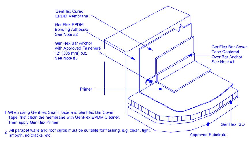
3. Polymer batten strips cannot be used for attachment into masonry wall substrates. Use only on smooth surfaces, e.g. wood or insulation.
