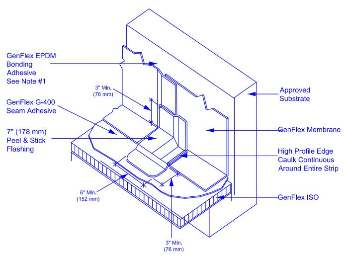
NOTE: All parapet walls and roof curbs must be suitable for flashing, e.g. clean, tight, smooth, no cracks, etc.
