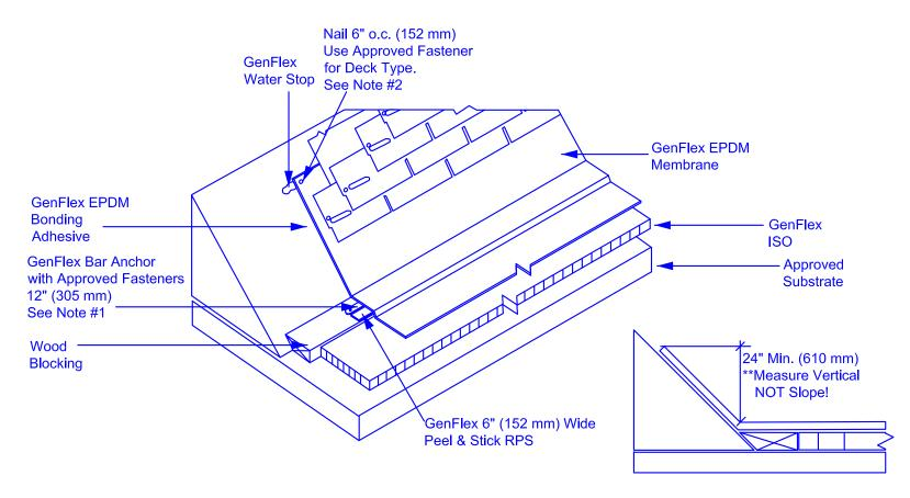
NOTE: EPDM Membrane must be extended as required to reach a point 24" (610 mm) above the finished roof surface. Top of membrane to be sealed to deck with bead of GenFlex Water Stop and be counter-flashed with roofing felt by a minimum of 3" (76 mm).
