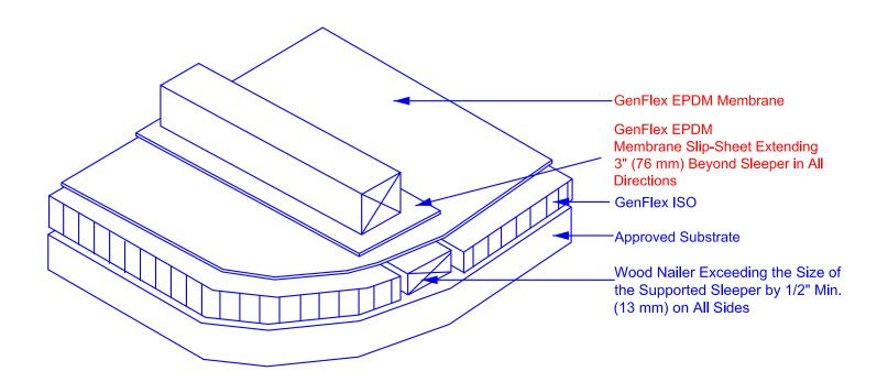
\* For use when the roof supported load exceeds 5 lb/in<sup>2</sup> (3.5 g/mm<sup>2</sup>). For loads less than 5 lb/in<sup>2</sup> (3.5 g/mm<sup>2</sup>), the sleeper may be set on a slip-sheet directly on the cleaned roof surface.
