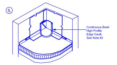
All parapet walls and roof curbs must be suitable for flashing, e.g. clean, tight, smooth, no cracks, etc. Polymer batten strips cannot be used for attachments into brick, block, or concrete wall substrates. Use only on smooth surfaces, e.g. wood or insulation.
