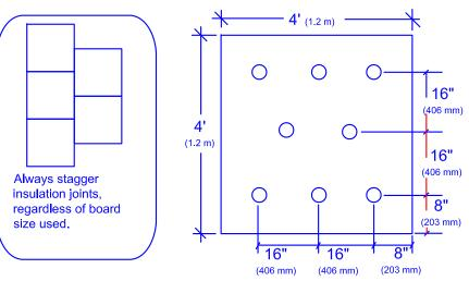
For use on buildings up to 50' (15 m) high. If building height exceeds 50' (15 m), contact the GenFlex Technical Department for an attachment pattern.
