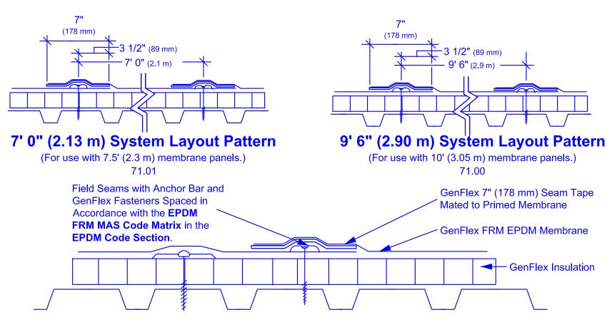
Position insulation and membrane sheets to enable securement into the top flutes on steel decks, ensure positive attachment, and reduce fastener movement. Insulation should be installed with board ends resting on the flute tops.
