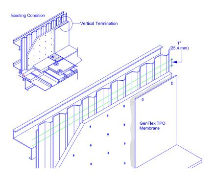
Cut a 1" (25 mm) strip out of the metal siding, starting at the upper edge of the purlin. Sand, prime, and paint the raw metal edge to prevent rust. Contact metal siding manufacturer for proper primer and paint types.
