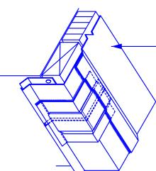
gravel stop metal. joint and extending to both edges of the reinforced TPO, centered over the metal Hot air weld a 6" (152 mm) wide strip of
