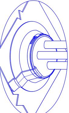
If the boot cannot be installed over the top of a penetration, the boot may be cut in order to place the boot around the object being sealed. If a cut is required, it must be overlaid and welded back together with TPO Non-reinforced Flashing prior to the boot being filled with GenFlex Pourable Sealer. Ensure the strip-in flashing extends a minimum of 1 1/2" (38 mm) beyond the step-off of the flange to ensure an adequate
