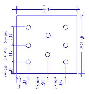
For use on buildings up to 50' (15.2 m) high. If building height exceeds 50' (15.2 m), contact the GenFlex Technical Department for attachment pattern.
