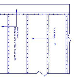
project must meet Factory Mutual criteria, refer to Detail roof. See the Mechanically Attached TPO Fastener width of up to 60% of the width of the field require half sheet perimeter securement. A half sheet T-42.04-3, and contact Factory Mutual for review. Matrix for fastener and spacing requirements. If the to the membrane securement used in the field of the panels may be used. Half sheet securement is equal All GenFlex EZ TPO Mechanically Attached Systems
