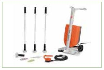
The InvisiWeld-S system consists of a specially coated 3" round plate that is used to both attach the insulation and the membrane through induction welding using the Isoweld® 3000 induction machine. This is available for use with .045, .060 and .080 GenFlex EZ TPO and EZ TPO Plus roofing membranes. It is FM Approved and is eligible for a GenFlex Roofing Systems Warranty for up to 15 years for .045 EZ TPO and 20 years for .060 and .080 EZ TPO membranes.
