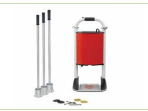
This high performance, non-penetrating TPO membrane fastening system utilizes a special TPO coated plate to attach an approved GenFlex insulation board to the roof deck. The GenFlex EZ TPO membrane is then laid out over the plates and induction welded to the back side of the TPO membrane using a heat induction welding tool.
