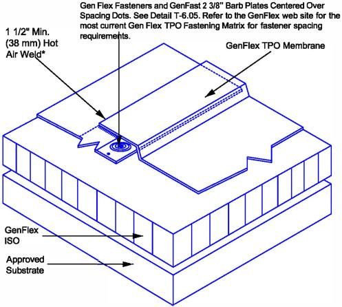
\*Position adjacent membrane panels on the factory-applied dashed reference line, and install membrane securement as required, centered over fastener and spacing dotted reference line.
