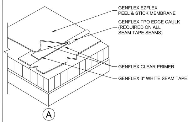
POSITION THE UPPER MEMBRANE PANEL AS REQUIRED TO ACHIEVE A 3" LAP OVER THE ADJACENT PANEL AND MARK THE POSITION OF THE UPPER MEMBRANE PANEL EDGE PLUS 1/4" (3 MM) WITH A CRAYON ON THE LOWER PANEL, PRIME THE SEAMING AREAS OF BOTH PANELS AND ALLOW THE PRIMER TO FLASH OFF, THEN POSITION AND APPLY THE 3" WHITE SEAM TAPE ALONG THE MARKS AS REQUIRED TO ACHIEVE 1/8" TO 1/4" (3-6 MM) OF EXPOSURE ONCE THE SEAM IS ASSEMBLED.
