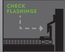
Check metal counter flashings at roof-to-wall transitions, and around rooftop units, vents and skylights. Resecure areas that are loose or have pulled away and re-seal as needed. PONDING WATER
