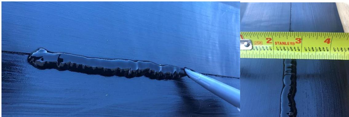
ACCEPTABLE GENFLEX PRIMER APPLIED UNDER SEAM AND UNDER SEAM2SEAM SEALANT
