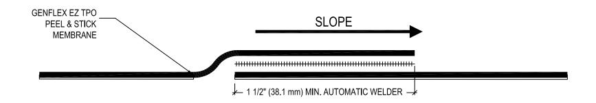
WHEN POLYESTER REINFORCEMENT OF TPO IS **EXPOSED, APPLY CUT EDGE TREATMENT TO** ENTIRE EXPOSED EDGE. REFER TO EZT-PS-LS-04.
