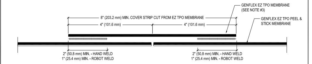
WHEN POLYESTER REINFORCEMENT OF TPO IS **EXPOSED, APPLY CUT EDGE TREATMENT TO ENTIRE EXPOSED EDGE. REFER TO EZT-PS-LS-04.**
