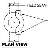
GENFLEX REQUIRES 4-1/2" (114.3 mm) TPO T-JOINT COVER OR TPO FLASHING (4" (101.6 mm) x 4" (101.6mm) MIN.) CENTERED OVER INTERSECTION OF SEAM.
