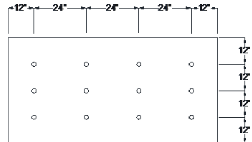
FM Global Fastening Pattern for 1-90 Attachment of GenFlex HD ISO Cover Board
